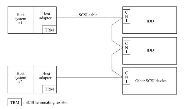
Figure 5.1 SCSI bus connections (2 of 2)
